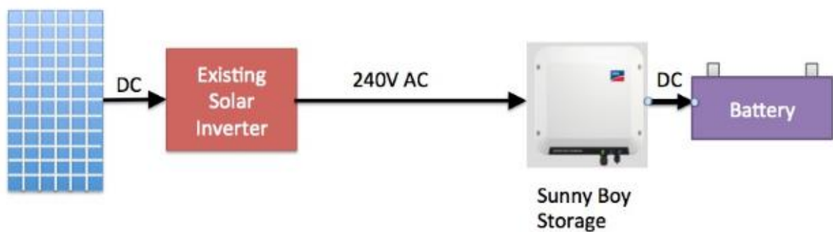
Figur 7 – Forenkla kopling inverter
